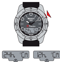
Select mode 12/24 hours – in 12 hour mode, the letter A (AM) or P (PM) appears between minutes and seconds when setting the time
