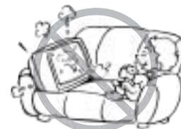
The slots and openings are provided to protect the TV from overheating and to help maintain reliable operation of the TV.
