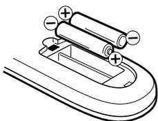
3. Close the battery cover on the remote control until the lock snaps.
