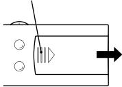
2 Install two "AA" size batteries. Match the + and – signs on the batteries to the signs on the battery compartment.
