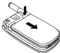
3. To remove the battery pack, lift up using the tab at the top of the battery.
