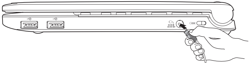
Figure 3-3 Connecting the adaptor to the computer
