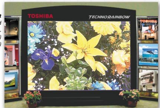
TR2006R flat 40 modules arranged 8 wide by 5 high. 3077mm (10.08 ft) by 1920mm (6.3 ft)
