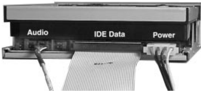
Cable Locations on Rear of DVD-RAM
