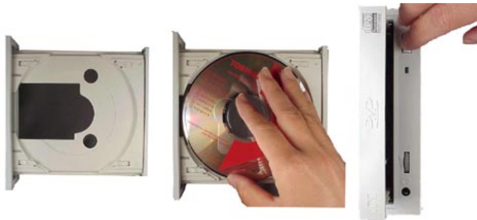
Figure 2. Inserting Disc Vertically
