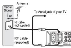
C: Receiving both DVB-T and ANALOG signal: If you need to receive both DVB-T and ANALOG signal (for hotels that send out cable and DVB-T signals together etc.), connect the antenna or cable to the ANTENNA IN (DVB-T) jack of this unit, and connect the ANTENNA OUT (DVB-T) jack to the ANTENNA IN (ANALOG) jack of this unit, then connect the ANTENNA OUT (ANALOG) jack to the
