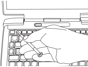
Using a flat-head screwdriver to pry off the panel
