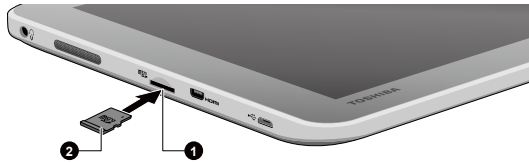
Figure 4-3 Inserting memory media (TOSHIBA WT8-B)
