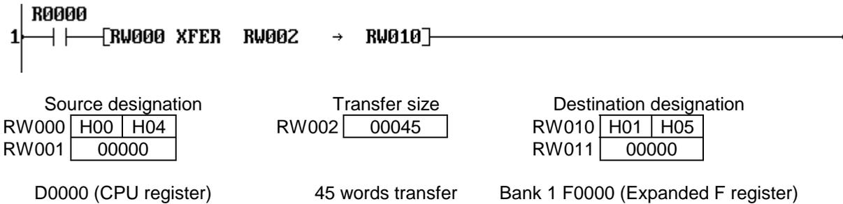
When R0000 is ON, 45 words data starting with D0000 is transferred to Bank 1 F0000 and after in the IC memory card.
