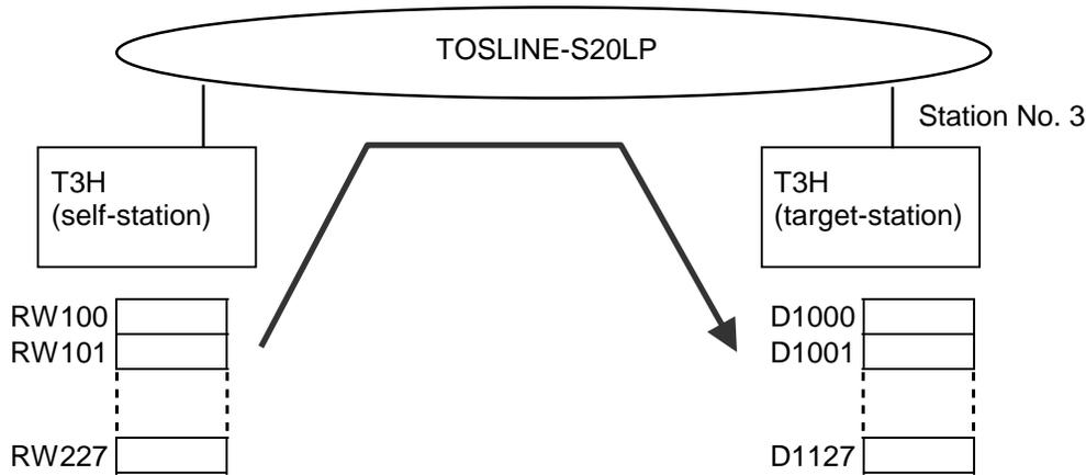
When R0020 is ON, 128 words data starting with RW100 is transferred to D1000 and after of the T3H on which station No. 3 S20LP is installed.
