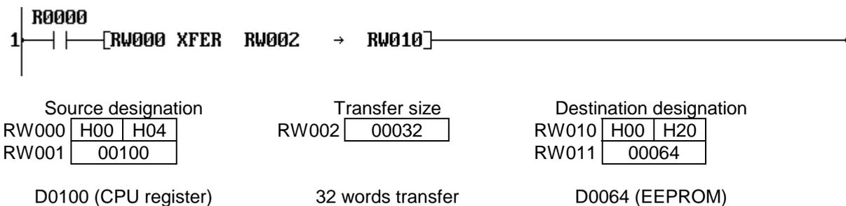
When R0000 is ON, 32 words data starting with D0100 is transferred to D0064 and after in the EEPROM. (Data write into EEPROM)
