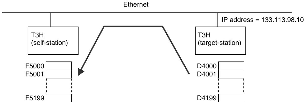
When R0030 is ON, 200 words data starting with D4000 of the T3H on which EN311 (IP address = 133.113.98.10) is installed, is read and stored in F5000 and after.
