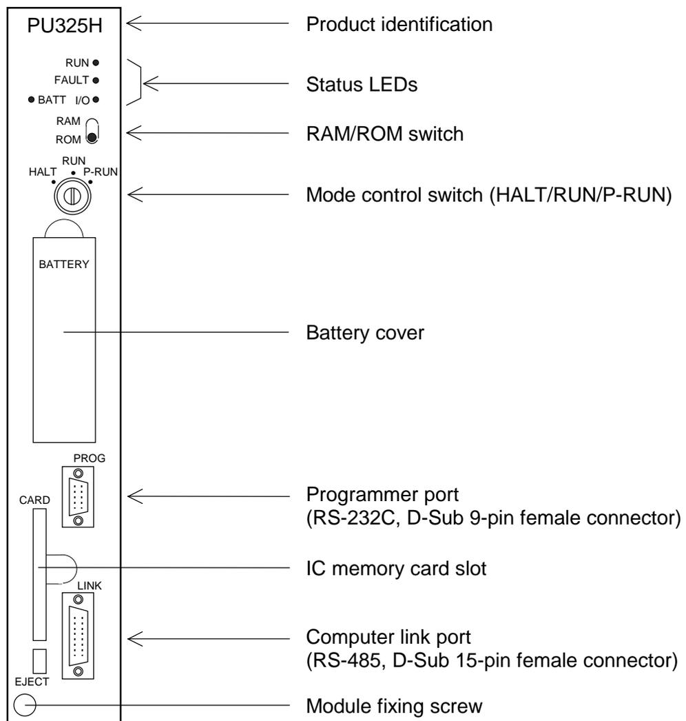
The external feature of the T3H CPU is the same as the T3 CPU except for the product identification.
