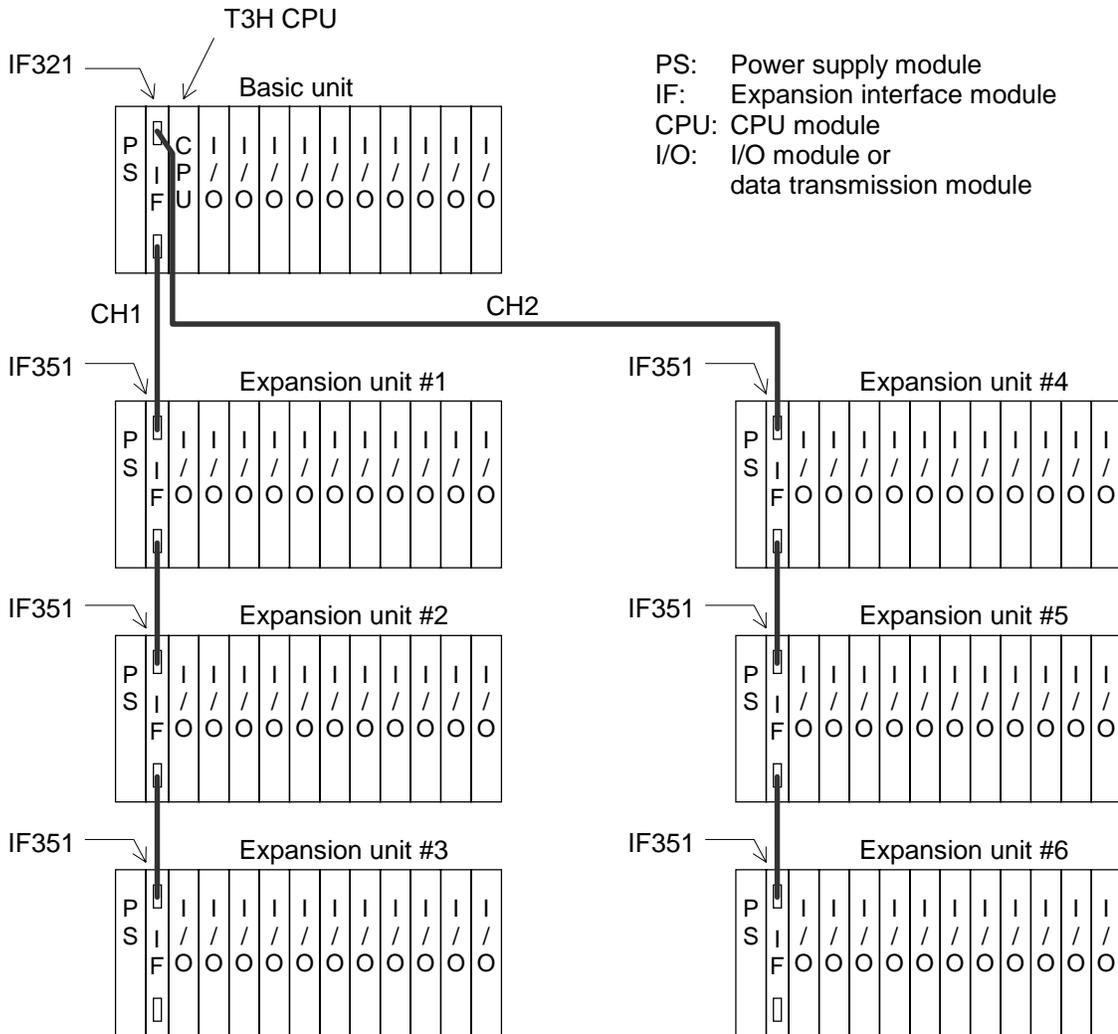
In this configuration, the T3H can handle up to 76 I/O modules. If 64 points I/O modules are mounted on all the I/O slots (76 slots), the T3H can control up to 4864 points of discrete I/O.
