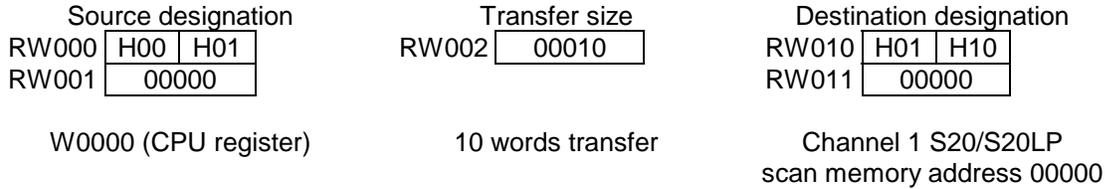
When R0000 is ON, 10 words data starting with W0000 is transferred to scan memory address 00000 and after of channel 1 S20/S20LP.
