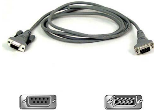
Figure 6: A Typical Serial Extension Cable
