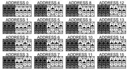
Address 0 is the FDP2 MASTER address. Address 1 to 15 are FDP2 SLAVE addresses that can be used to create large control groups.
