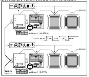
The MASTER FDP2 can be configured using SW1 and SW2 to operate using one of the three preset modes Heat, Cool or Auto. Alternatively the MASTER can be configured for local control, in which case the remote controller attached to the MASTER FDP2 can be used to set the operating settings during master duty.
