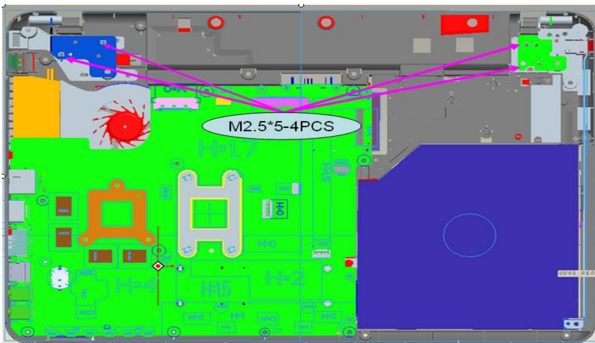
Figure 4-8-8 Securing the hinge screws
