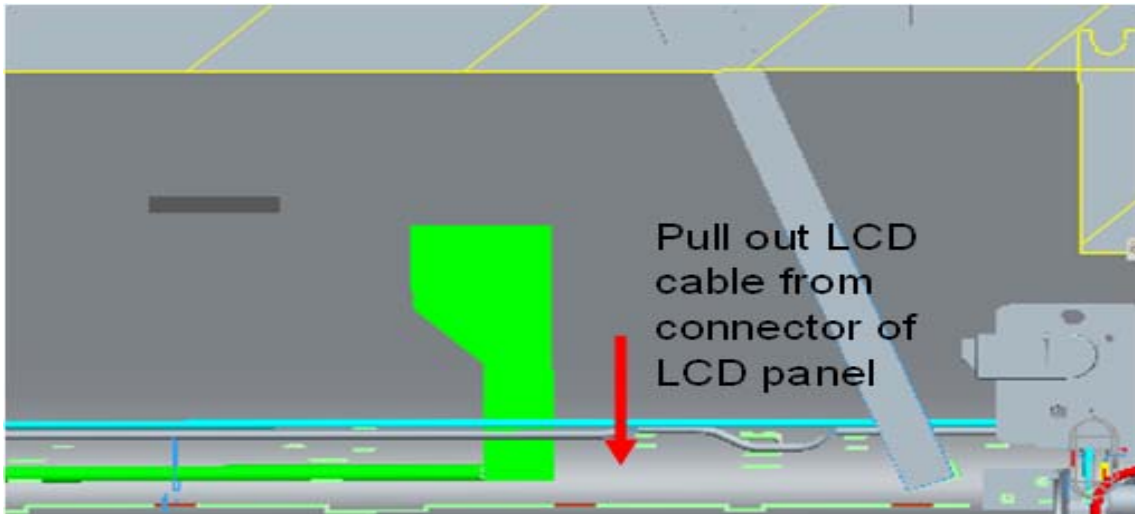
Figure 4-8-6 Remove the LCD cable from LCD panel
