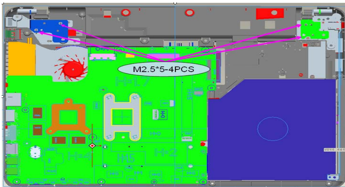
Figure 4-8-7 Remove the hinge screws
