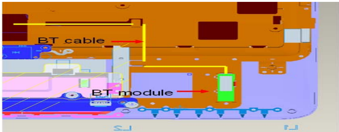
Figure 4-19-1 Remove the Bluetooth cable
