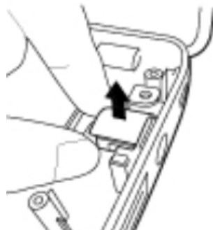
Figure 4-33 Removing DC in cable
