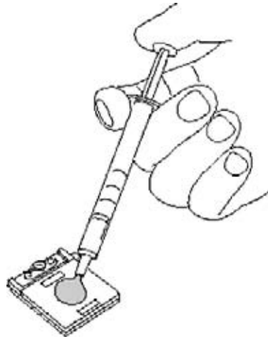
Figure 4-35 Applying new grease
