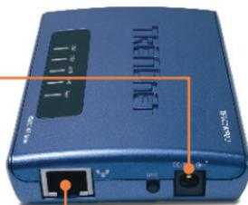
3. Connect a RJ-45 network cable from a Switch/Router to the **LAN** port of the Print Server.
