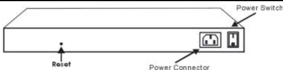
Figure 4. Rear panel of the Switch
