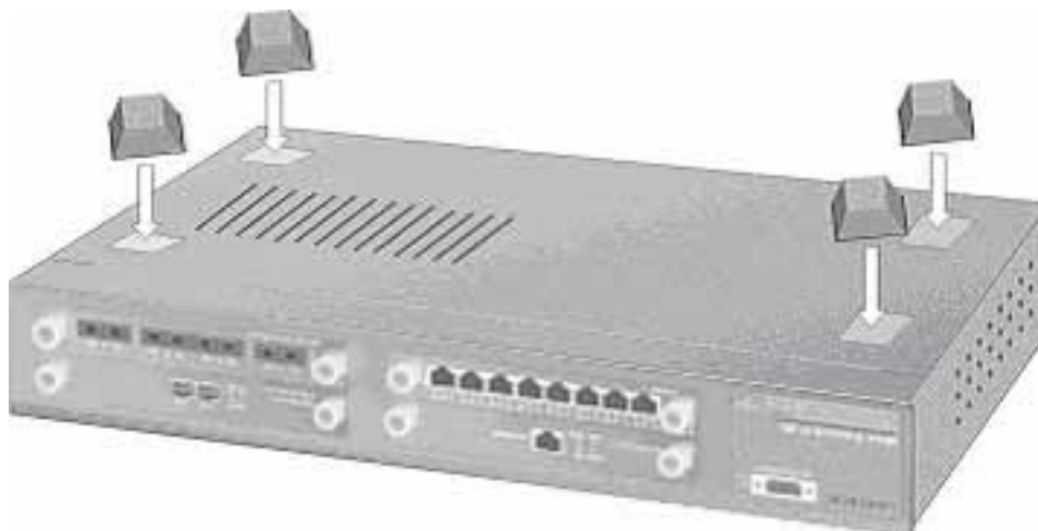
Figure 4-1. Attaching Rubber Feet to each corner on the bottom of the Switch
