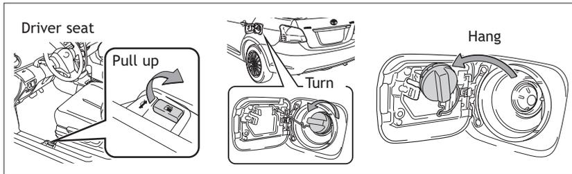
**NOTE:** Tighten until one click is heard. If the cap is not tightened enough, Check Engine “
