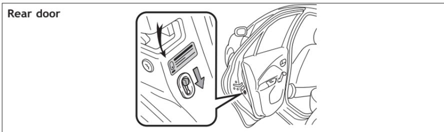
Moving the lever to “LOCK” will allow the door to be opened only from the outside.
