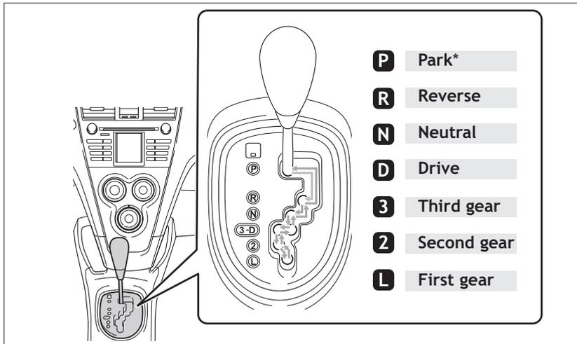
\* The engine switch must be "ON" and the brake pedal depressed to shift from Park.
