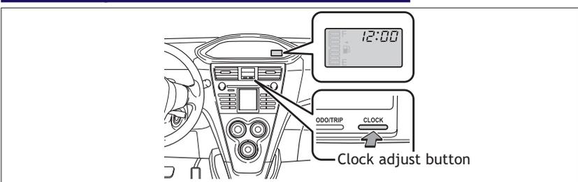
(1) Push and hold the CLOCK button to enter adjustment mode. (2) Press CLOCK button to adjust hours. (3) Wait five seconds to adjust the minutes. (4) Wait another five seconds for process to complete.
