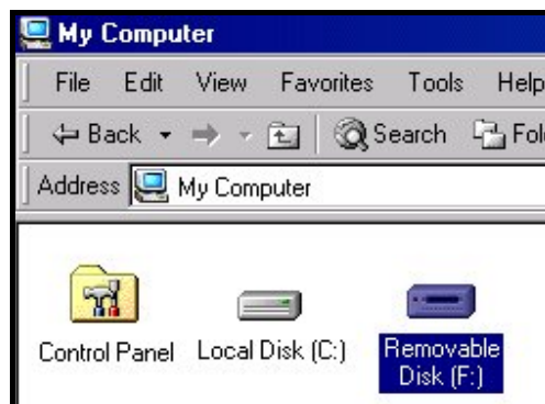
Figure 6. The MP320 shows up as a Removable Disk in the My Computer window
