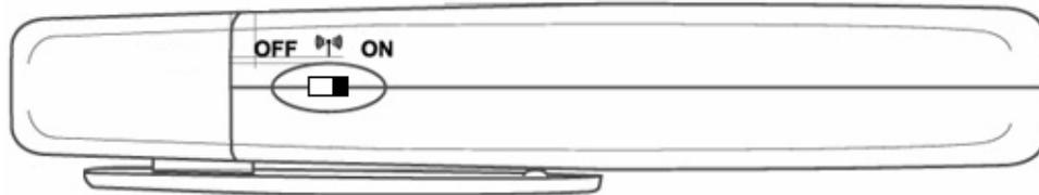
When the switch is set to the “ON” position, you can write/read data to/from your **JetFlash** and simultaneously use it for wireless applications. When the switch is set to the “OFF” position, you can write/read data to/from your **JetFlash**, but the wireless function is disabled. Please set the switch to the “ON” position before using the Wireless LAN function of your **JetFlash**.
