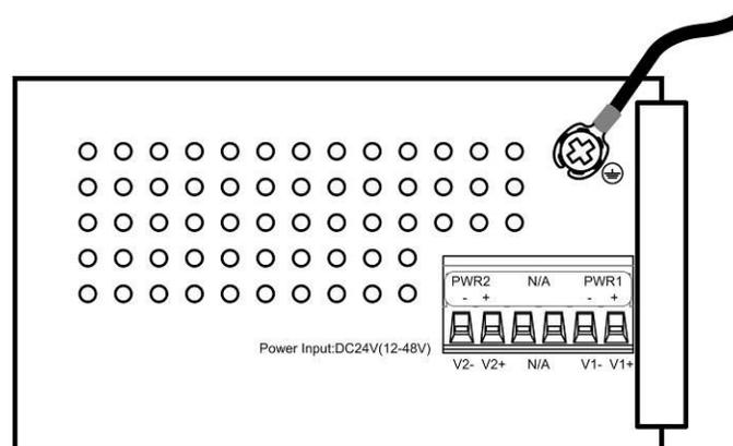
**Figure 7: Industrial Switch Ground Screw (Bottom Panel)**
