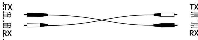
2. Connect cable with connector installed at TX location on media converter to RX location on attached device.
