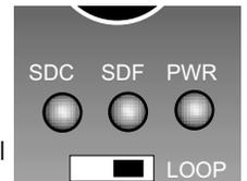
**SDF** **Signal Detect/Fiber** - Steady LED indicates fiber link is up.
