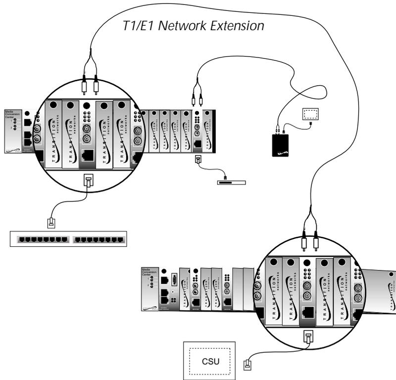
NOTE: T1/E1 MEDIA CONVERTERS MUST BE USED IN PAIRS. A TRANSITION Networks CSDTF10xx chassis media converter can be used with another CSDTF10xx chassis media converter, a SSDTF10xx stand-alone media converter, or with a previous model TRANSITION Networks T1/E1 media converter, such as a C/T1E1-CF-01 or a T1E1-CF-01.
