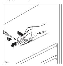
Unscrew the light cover and then pull it outward by pressing as shown in the figure. Unscrew the bulb and replace it with a new 15 watt bulb (available from your nearest Service Force Centre).
