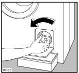
Unscrew and remove the filter.
