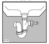
Push the drain hose onto the spigot and secure with a clip if required, ensure a loop is formed in the drain hose (see diagram) to prevent waste from the sink entering the washin machine.
