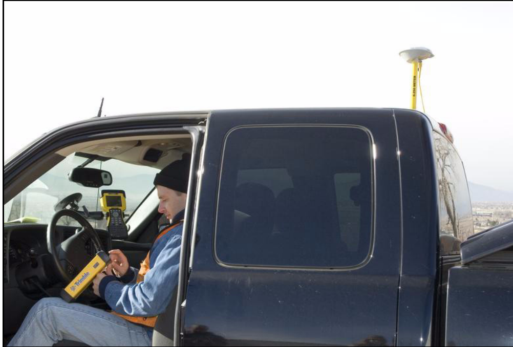
Figure 5.5 Configuring an SPSx51 from the cab. A Zephyr Model 2 antenna is mounted on the roof.
