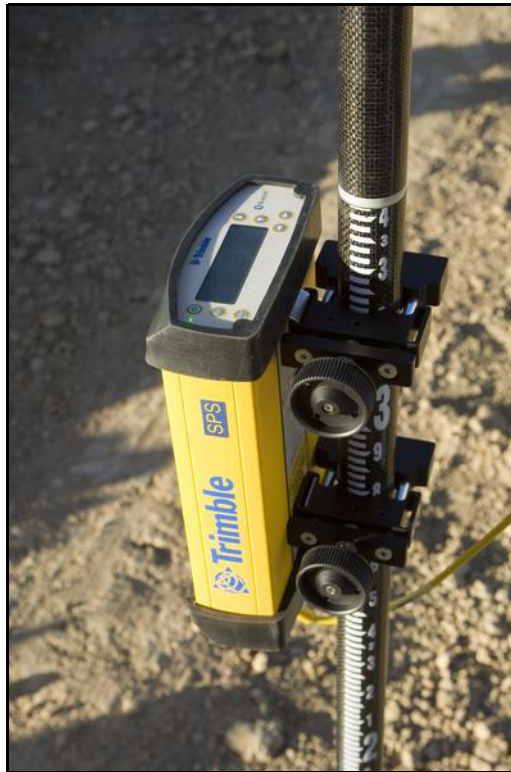
Figure 4.1 Rod mount for a modular GPS receiver
