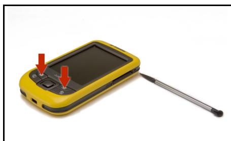
Figure 2.8 Resetting the handheld to factory default settings
