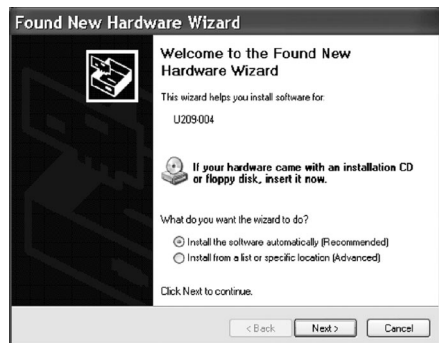
Figure 1 - The Found New Hardware Wizard launches automatically when you first plug in the USB-to-Serial adapter.
