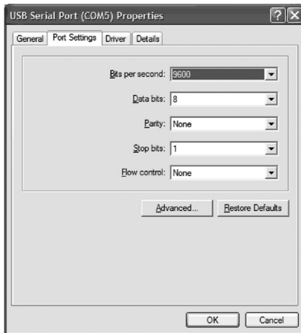
Figure 16 - USB Ports Settings box, which lets you set the default port settings, view the advanced options, and restore the default settings.
