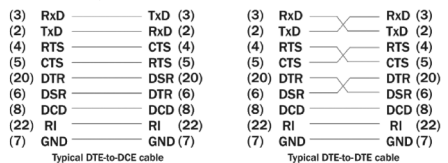
Figure 13 - illustrates the RS232 pinouts for typical DTE- to-DCE and DTE-to-DTE cables with 9-pin connectors.
