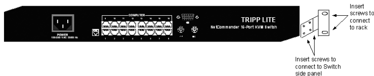
Figure 7 Connecting the L-shaped bracket
