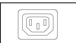
**Secondary AC Input Power Inlet (Model PDUMH15ATNET):**
