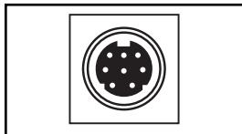
**Mini-DIN Serial Port:** Use this port to provide a direct terminal connection to a computer with a terminal emulation program. A serial cable (part number 73-1025) is included with the PDU. If you need to order a replacement cable, contact Tripp Lite Customer Support at (773) 869-1234.
