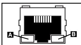
**Ethernet Port:** Use this RJ-45 jack to connect the PDU to the network with a standard Ethernet patch cable. The Link LED **A** and Status LED **B** indicate several operating conditions, as shown in the table below. *This port is not compatible with PoE (Power Over Ethernet) applications.*
