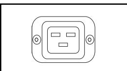
**Secondary AC Input Power Inlet (Model PDUMH20ATNET):**
