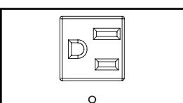
**NEMA 5-15R Outlets (Model PDUMH15ATNET):** During normal operation, the outlets distribute AC power to connected equipment. When an outlet is live, the associated LED illuminates.
