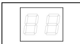
**Digital Load Meter (Ammeter):** The total electrical current used by the PDU is displayed on the digital meter in amperes.
