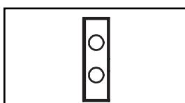
**Input Source Indicator:** When the PDU is connected to a live AC power source, the Primary or Secondary input LED illuminates to indicate which source is supplying power to the PDU outlets.
