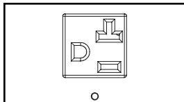
**NEMA 5-15/20R Outlets (Model PDUMH20ATNET):** During normal operation, the outlets distribute AC power to connected equipment. When an outlet is live, the associated LED illuminates.
