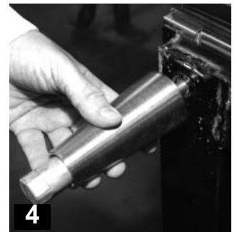
4 Thread leg into cabinet bottom frame rail.
