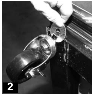
2 For leveling, insert the shim between the castor and frame rail.
