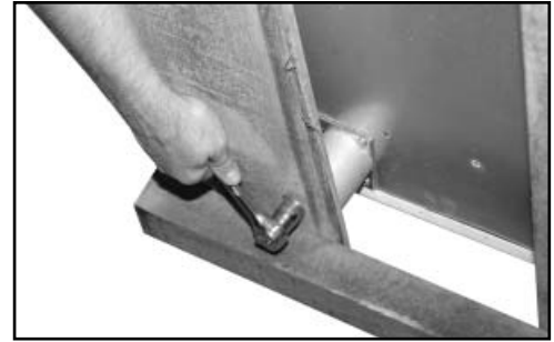
Removing skid from bottom of cabinet.
