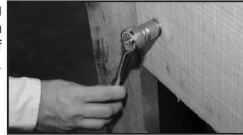
Removing skid from bottom of cabinet.
