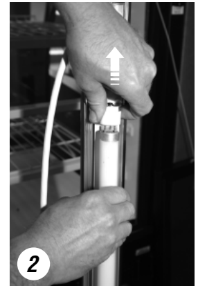
2 Remove bulb by gently pulling up on spring loaded lampholder.
