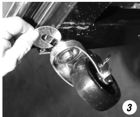
Use shims as necessary to level cabinet.
