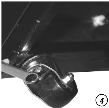
Tighten castor in position with castor wrench.
