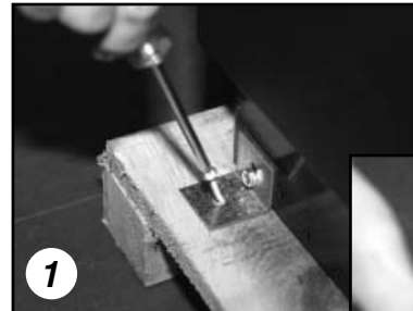
1 Removing bracket from skid.
