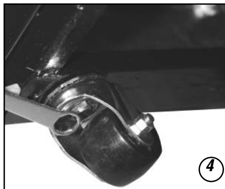
Tighten castor in position with castor wrench.
