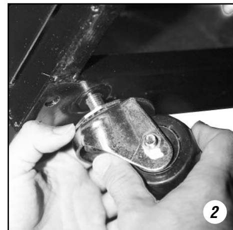
Thread castors into existing leg leveler holes.
