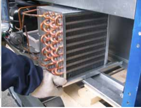
Pull out the condensing unit
