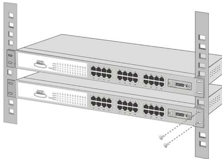
Figure 7. Mount the Switch in an EIA standard 19-inch Rack
