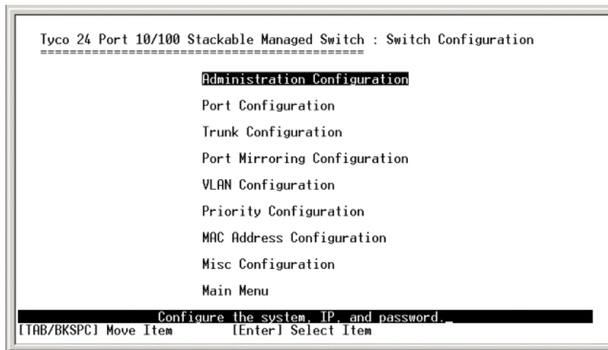
Figure 16. Switch Configuration Screen
