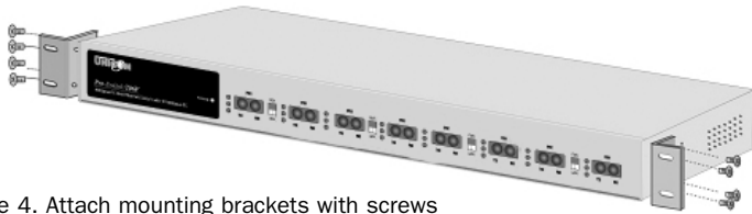
Figure 4. Attach mounting brackets with screws
