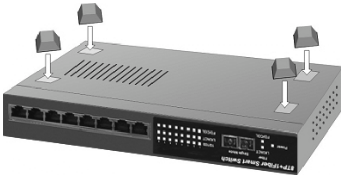
Figure 2-6. Attaching Rubber Feet to each corner on the bottom of the Switch
