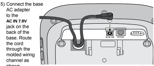
to the **AC IN 7.8V** jack on the back of the base. Route the cord through the molded wiring channel as shown.
