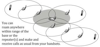
If you want to use the repeater with a new base, simply register the repeater to the new base (see page 37). The repeater overwrites its own link to the base.
