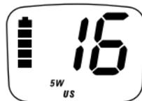
Level 0: The radio cannot transmit. If the battery level drops to level 0 during transmitting, the transmission will be canceled.
