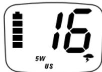
**3** When the unit receives a warning signal, it beeps for 5 seconds.
