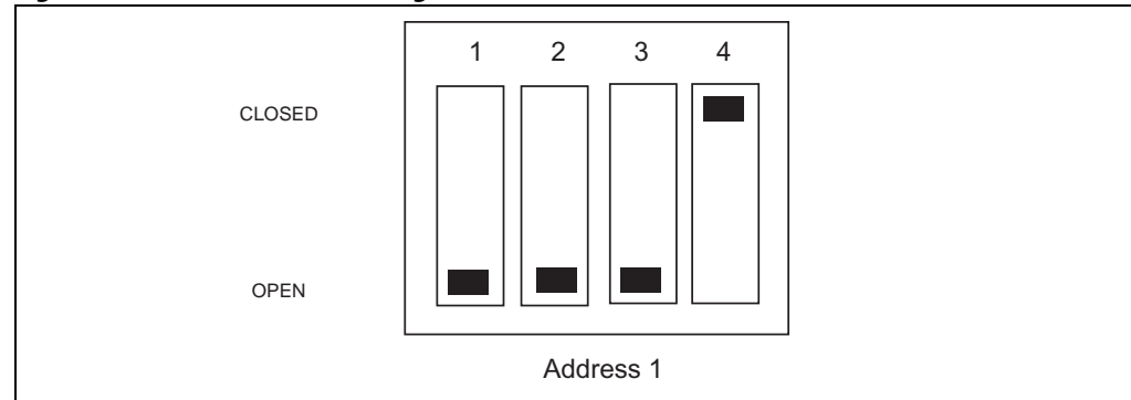
Figure 5-2: Switch SW-1 setting for ID 1
