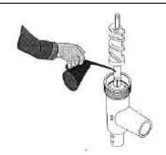
The shaft of the feed screw should be lubricated with grease before the feed screw is inserted into the housing. Use e.g. paraffin oil or castor oil, never salad oil.
