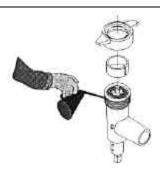
The thread of the housing should be lubricated with grease before the distance ring and the ring are mounted. Use e.g. paraffin oil or castor oil, never salad oil.
