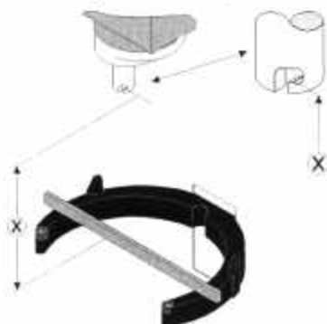
fig.7a Measuring of bowl height:
