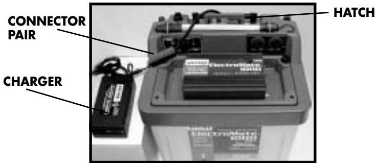
FIGURE 8 – BATTERY CHARGER HOOKED TO ELECTROMATE
