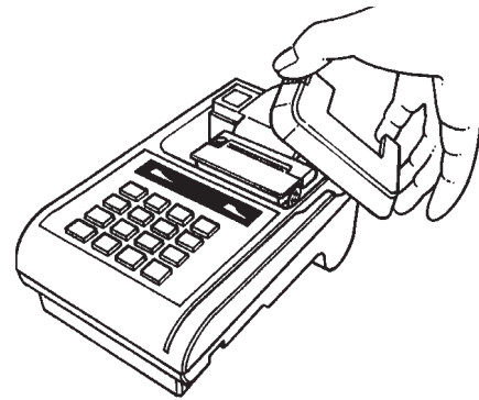
Figure 3-3. Removing the Printer Cover
